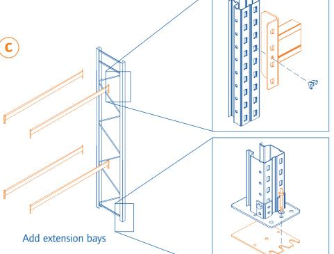
Fit safety pin through beam connector and post
